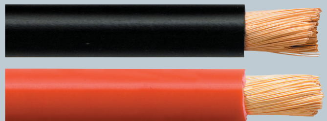
Flexible Battery/Starter Cable - 60 mm 2 475/0.40 mm. 415 amp.
